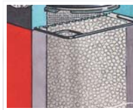
Snow Storm filled to prevent fluidization and channelling
